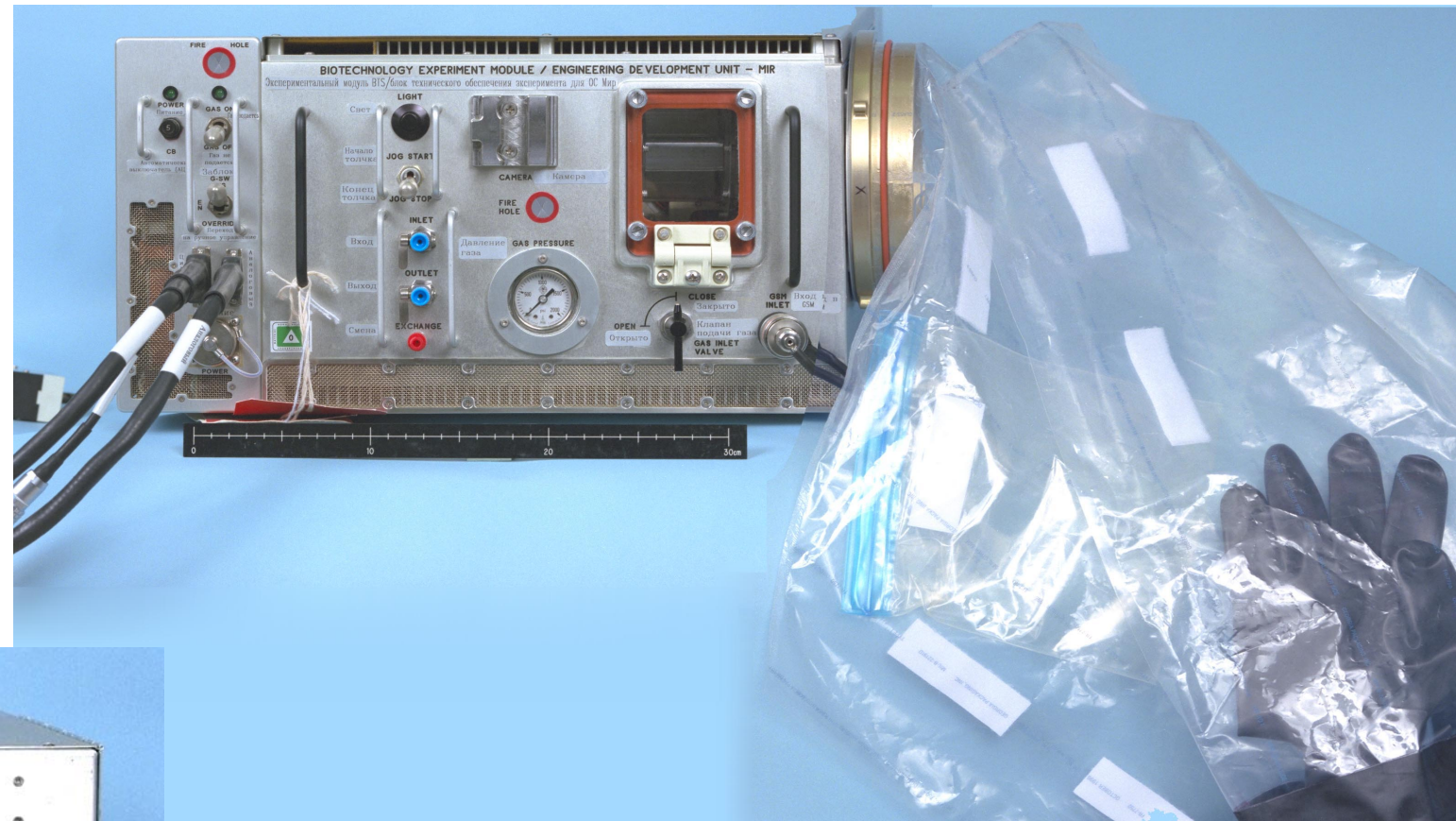
Figure MG-99 EDU-M Front with Glove Bag Attached (Note That the "X" on the Ring is Facing Front.)
