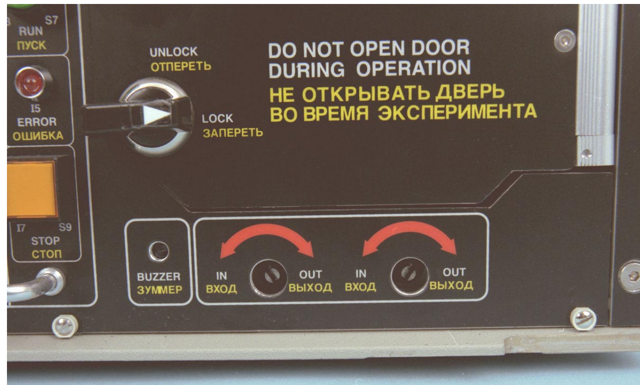
Figure MG-346 QUELD Sample Adjusters Used to Manually Insert or Remove Samples
